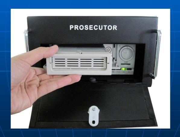
Put the HDD rack into the USB removeable mobile rack and connect to the USB port of PC or labtop that install HDD Viewer after that run the HDD Viewer program.
