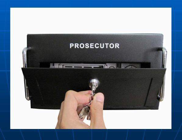
Turn off the HDD mobile rack key and pull out the HDD rack.
